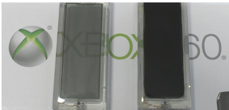
Figure 2.1: **Light blocking with LCDs.** Left: unpowered and transparent, right: powered and opaque. Although the powered LCD [Ama] appears opaque the intensity of the infrared laser is not degraded enough for blocking.
