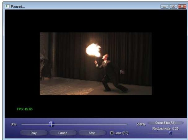
Figure 3. The graphical user interface of the free viewpoint video player. Resembling to a standard media player interface with play, pause and stop buttons as well as a progress bar, our player provides additionally the possibility to adjust the playbackrate. By dragging the left mouse button, the viewpoint can be changed interactively.
