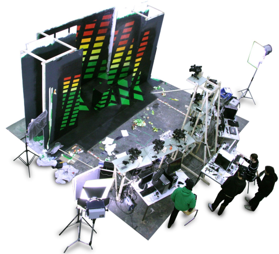
Figure 1: "Who Cares?" set. Eleven HD camcorders captured various graffiti motifs. With our approach we are able to synthesize novel spatial and temporal in-between viewpoints.
