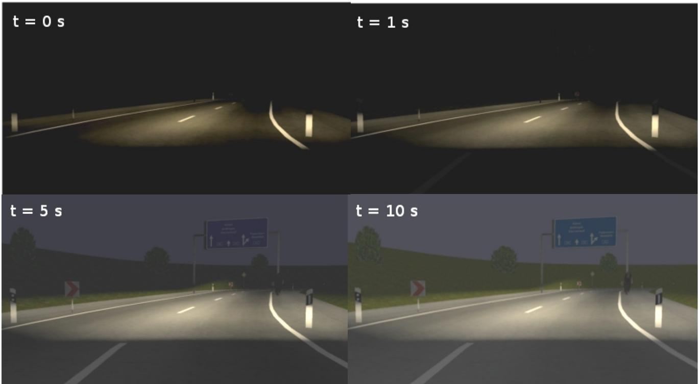
*Figure 9: Screenshots of the driving simulation with integrated glare handling. After a glare, the scene is darkened abruptly. It is then relit over time, based on the measured contrast perception.*
