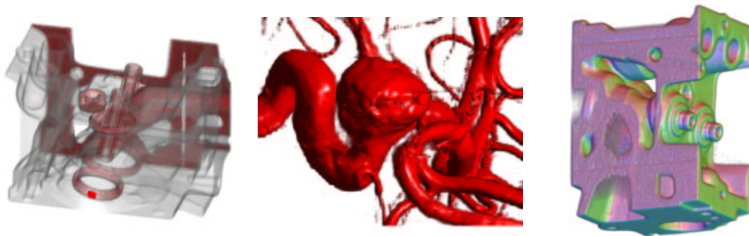
Figure 1: Real-time volume rendered images enabling classification and phong shading in single pass rendering on GeForce3. From left to right: Gradient magnitude modulation, zoomed view of aneurism, and differently colored light sources.
