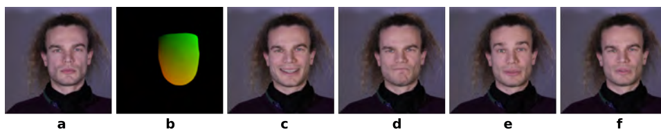
Figure 4.5: This figure demonstrates how the different facial expressions look like after rendering the reenactments. For an input video (a) the facial expression is altered with the emotions happiness (c), disbelief (d), positive surprise (e) and disgust (f). For this a neural renderer is used on the uv maps (b) of the manipulated face meshes.
