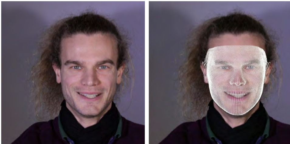
Figure 4: Illustration of the full face mask that is found automatically in every single frame of the input video.
