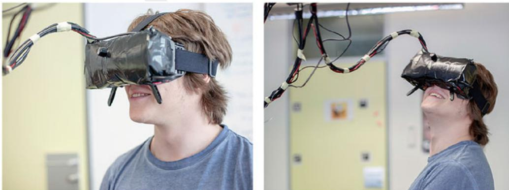
**Fig. 4** Our experimental setup: A participant is watching an immersive video using our custom-built head-mounted display with integrated eye tracking. The participant is seated on a rotatable chair, in order to allow safe and free  $360^\circ$  body and head movement
